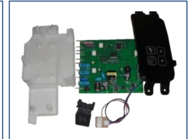
PCB, housing, humidity sensor with bracket
