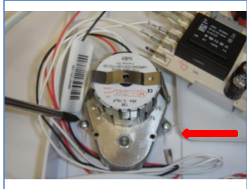
Loosen the two screws with geared motor
