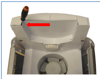
Place the unit upside down and resolve on both sides
