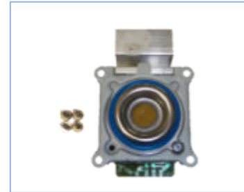
Nebulizer with gasket. CAUTION: When changing the nebulizer, don't forget the gasket
