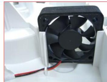
CAUTION: Put the fan-cable at the assembling in it's forseen port
