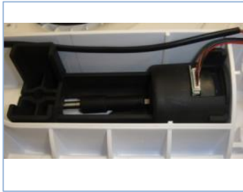
Remove gear motor
