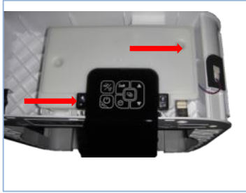
Loosen the 2 screws of the print and the housing
