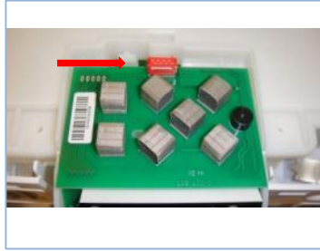
Remove the red cable and the cover
