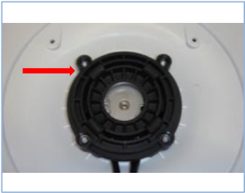
Remove the 4 screws of the fan motor cover
