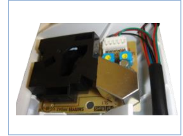
Remove particle sensor
