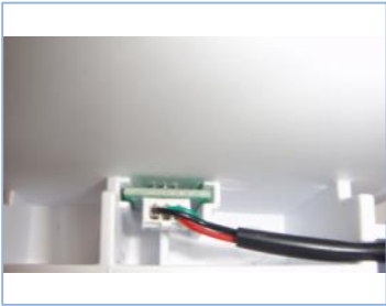
Remove the water level sensor
