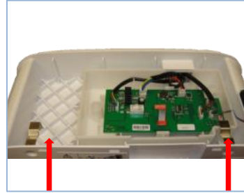
Remove the cable, the print and both contact plates. CAUTION: Do not forget the contact plates when assembling
